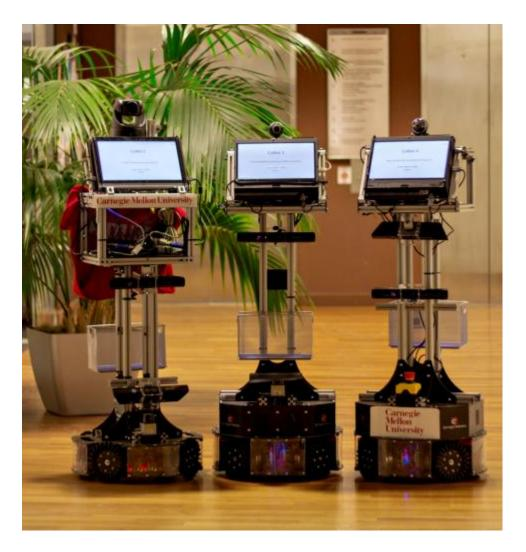
Three of the autonomous mobile CoBots developed at Carnegie Mellon University (Carnegie Mellon University)
